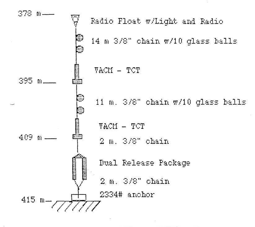
USGS MOORING R9 WINTER DEPLOYMENT bottom tripods were deployed within 200 m of the VACM moorings at sites R-8 and PJ-1. All deployments proceeded smoothly in large part because of the large, stable platform provided by the M/V Farnella, the bow thruster propulsion, and the experience of the ship's crew.
