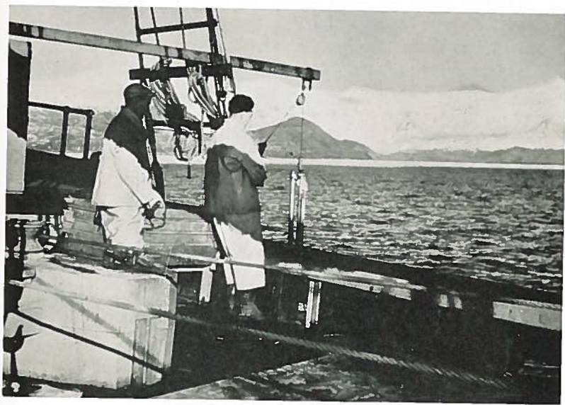
FIG. 49.—Taking the temperature and sampling the water at Stepovak Bay. This snow-rimmed body of water was not as cold as one might think. At 7 o'clock in the morning, October 25, the surface registered 5°41 C. (41°74 F.). Near the bottom, 22 fathoms down, the water was warmer, 9°90 C. (49°64 F.).
