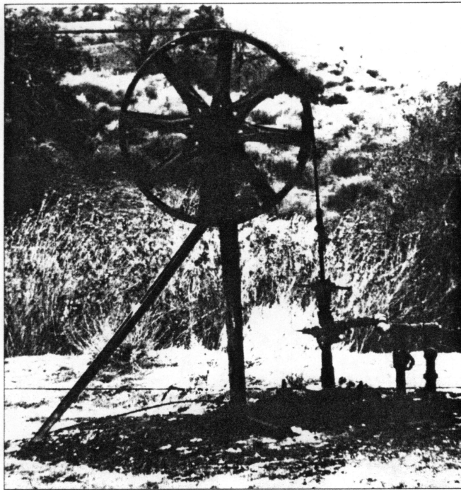
Figure 3. A turn-of-the-century oil-well pump, used until recently on the Marr Ranch, northeastern Simi Valley. Photograph by R. L. Squires.
