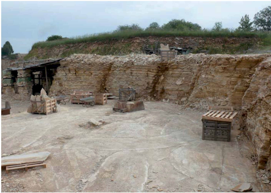
Fig. 4. Typical quarry in the Eichstätt district, where the platy Upper Jurassic Solnhofen Limestones (Eichstätt Formation, lower Hybonotum Zone) are quarried for floor and roof tiles.
