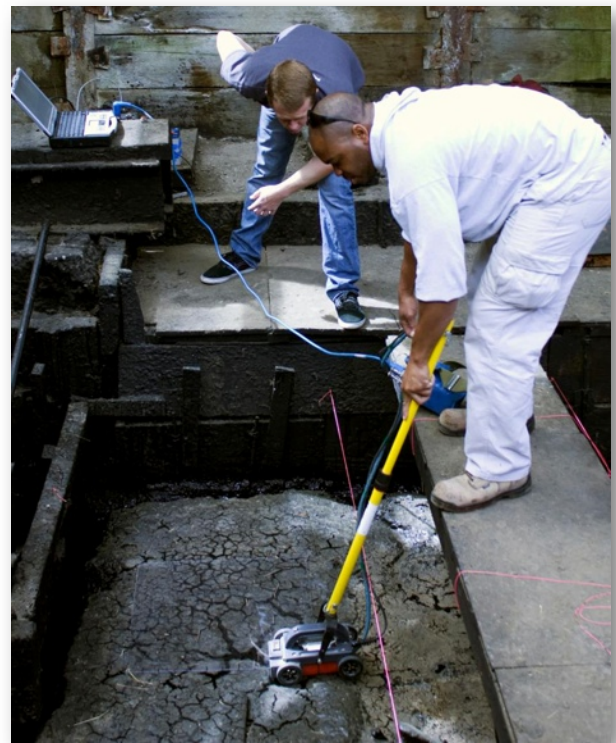
Staff from GeoVision using GPR in Pit 91.
